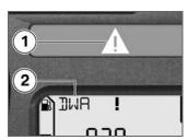
Anti-theft alarm warning are shown as warnings **2** in conjunction with the general warning light **1** following the pre-ride check and refer to the capacity of the internal anti-theft alarm battery.
